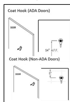
Coat Hook & Bumper Dimensions
